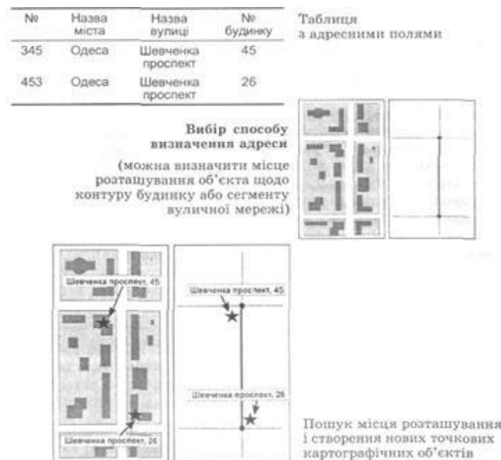
Fig. 11. Geocoding the location of buildings by address binding in the StreetMap database
