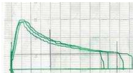
Fig. B1. Alveogram of the dough sample without additives (control)
