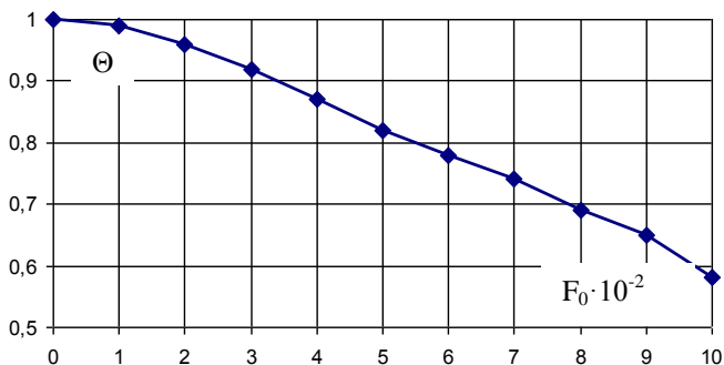
Fig. 6. Dependence of Fourier's criterion on relative temperature during heat processing of eggplants
