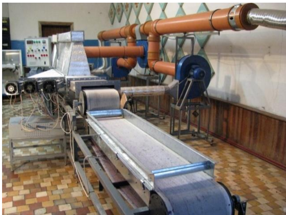
Figure 2.1 Equipment for seed irradiation with MWF of EHF developed by Kharkiv National Technical University of Radio Electronics, installation of a microwave design of the “UMVK-1” brand
