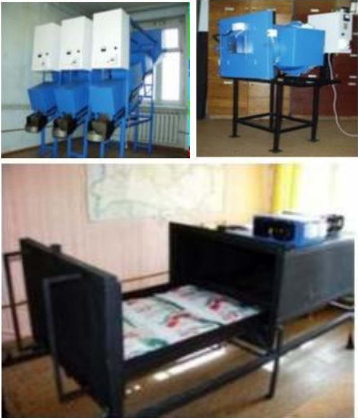
Figure 1.4 Installations for pre-sowing seed treatment, drying and disinfection with MWF of EHF
