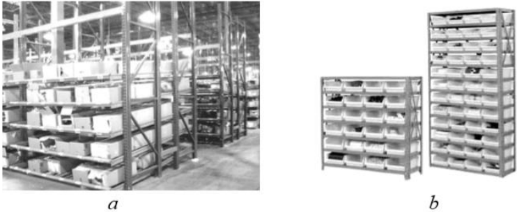
Fig. 2. Types of storage modes: a – carton flow rack; b – bin shelving
