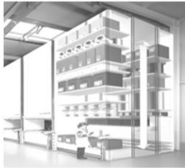
Fig. 5. Vertical lift modules
