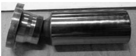
Fig. 1 – Piston with pivot of axial hydraulic pump
