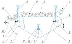
1 -load-carrying belt; 2,3 -supporting rollers; 3 -valve; 4.5 -moving shafts; 6 -vibration exciter; 7 -tension device; 8 -elastic supports; 9 -feeding tray; 10 -unloading tray; 11 -elastic element; 12 -adjustable nut; 13 -products; 14 -finely dispersed ice; 15 -tray for removal of snow fur particles.
