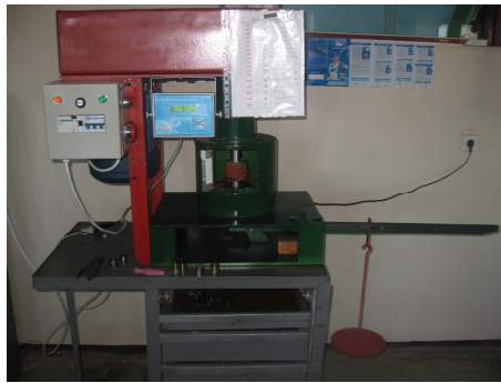
Fig. 3. Appearance of a friction machine
