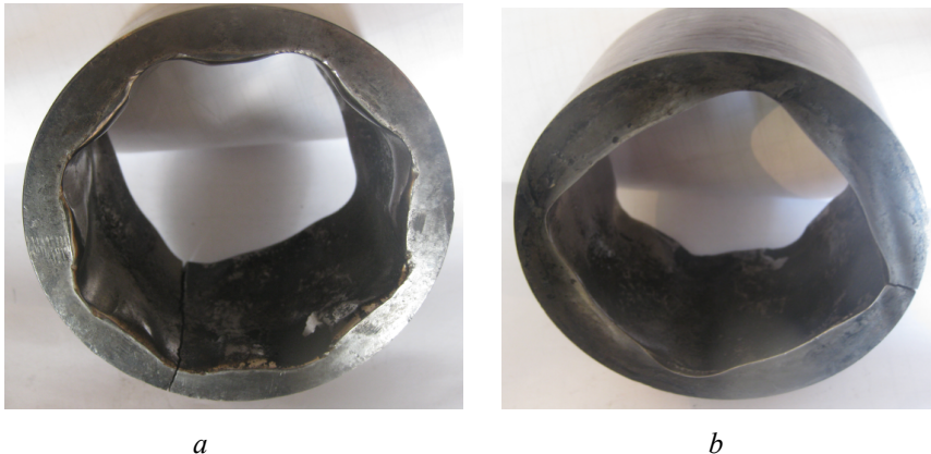
Fig. 2. Photo of a worn die: (a) in front and (b) behind
