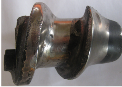
Fig. 1. Photo of a worn shank of extruder screw
