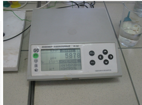
Fig. 5. Laboratory microprocessor ionometer I-160 M
