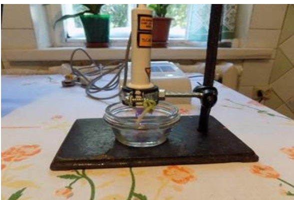
Fig. 1. Image of the process of laser treatment of the root system of beans "Saharnaja"
