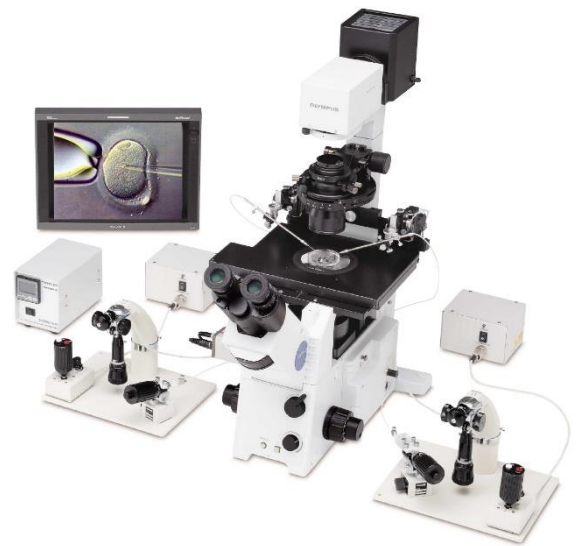
Fig. 4. An automated system for microsurgery of the cell, including an inverted microscope, motorized micro-tool holders, micro-pumps and a video monitoring device
